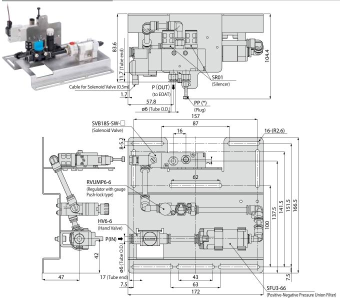
\*) when using with double-acting grippers, remove the plug (PP) and install piping.
