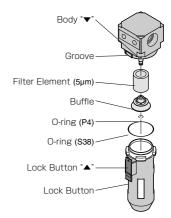
2) 0.3 and 0.01µm Element (FTD300-□-□D、FTM300-□-□D)
